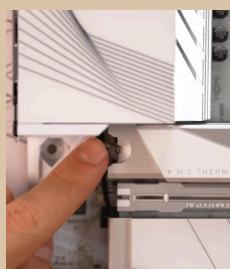
Unscrew the cover of M.2 slot (image on the right), newer motherboards tend to have a latch, which needs to be flicked (picture to the left), peel the plastic covering the thermal paste on cover and the heat shield. You might need to buy your own heat shield if it's not included on the slot.
