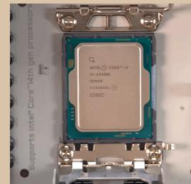
Pull down the cover onto the CPU after ensuring the CPU is seated properly and secured without damage. If done correctly, the cover should come off.
