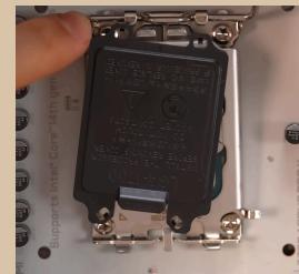
After pulling down the cover onto the CPU, pull down the latch back into its original place to lock the CPU in place.
