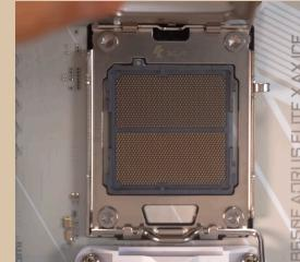
Align the triangles and gently place the CPU on the socket, gently push along the sides into place. Do not apply force, it will cause damage to the pins.
