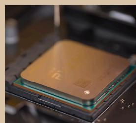
After inserting CPU in the Socket, pull down the lever to lock it into place, you may feel resistance when you do it for the first time
