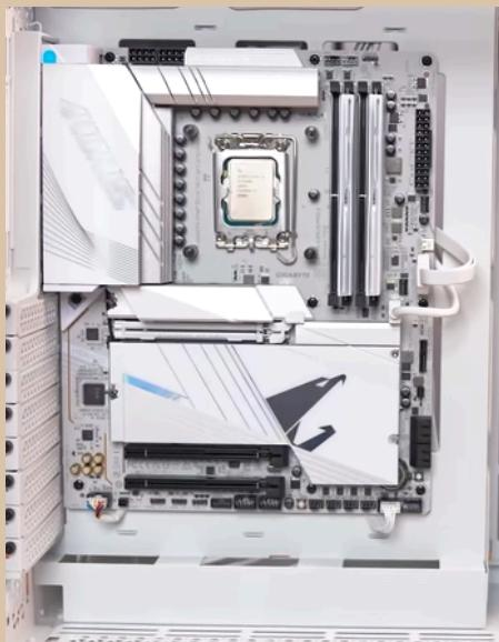
Please refer to the motherboard and the case manual to plug in all the case ports in the front/top to the motherboard. Notably, USB 3.0, USB C, USB 2.0, HD Audio, 3 PIN-RGB, JFP1 Connectors (Power, Restart, Shutdown), please note that all these ports may or may not be present.
