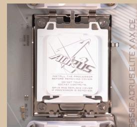
After pulling down the cover onto the CPU, pull down the latch back into its original place. If done correctly the cover should come off.
