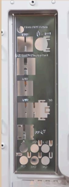
Insert the IO shield onto the case, IO shield is a cover which covers your usb ports on the motherboard, some motherboards have them built onto it, for ones which don't, find the IO shield in the motherboard box and insert it onto the rectangular opening behind the case.
