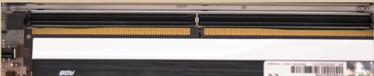
Place the stick on the slot and push it into place, if done correctly the tabs should lock it into place.
